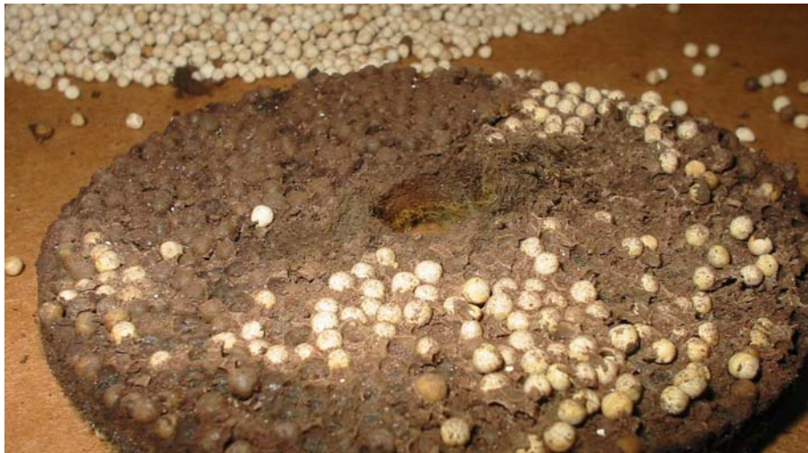
Reduced desiccant levels mean less margin for error when moisture creeps into the receiver drier.
